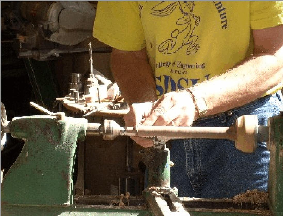
A bead is rolled next to the tenon on the end of the spindle. The other end of the square blank is driven in a shop made socket on a small faceplate.
