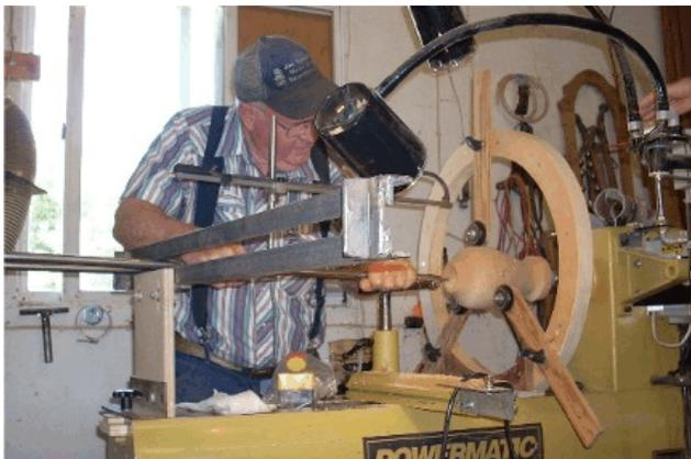
Jim demonstrating a system for deep boring and support of the work
